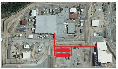
LANL TA-55 complex with proposed underground production modules shown in red. PF-4 is the large central structure; RLUOB at lower right.
