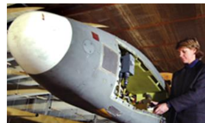
Sandia National Laboratories performing electromagnetic qualification measurements on the air-launched cruise missile.
