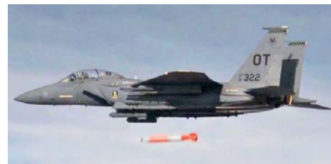
An F-15E drops a B61-12 test unit during a development flight test.
