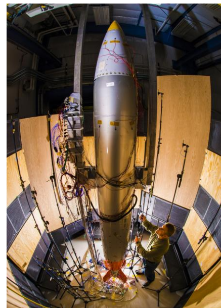
Mechanical engineer adjusts a microphone for an acoustic test on a B61-12 system. The unit is surrounded by banks of speakers that expose it to an acoustic field. The sound pressure reaches 131 decibels, similar to that of a jet engine.
