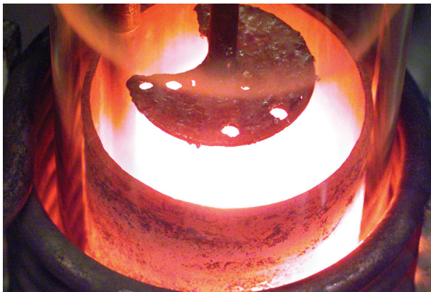
Figure 2.2: Molten plutonium in a crucible. Before the Laboratory's cast pits could enter the stockpile, the Laboratory needed to verify that their quality and performance equaled or exceeded the quality and performance of the wrought pits produced at Rocky Flats.
