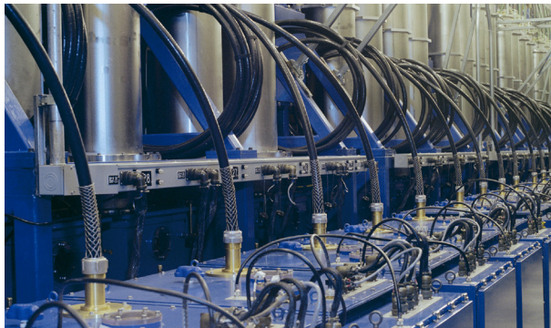
Figure 3.9: The Laboratory built DARHT to position two massive x-ray machines perpendicularly to capture two- and three-dimensional images of materials imploding at speeds greater than 10,000 miles per hour.
