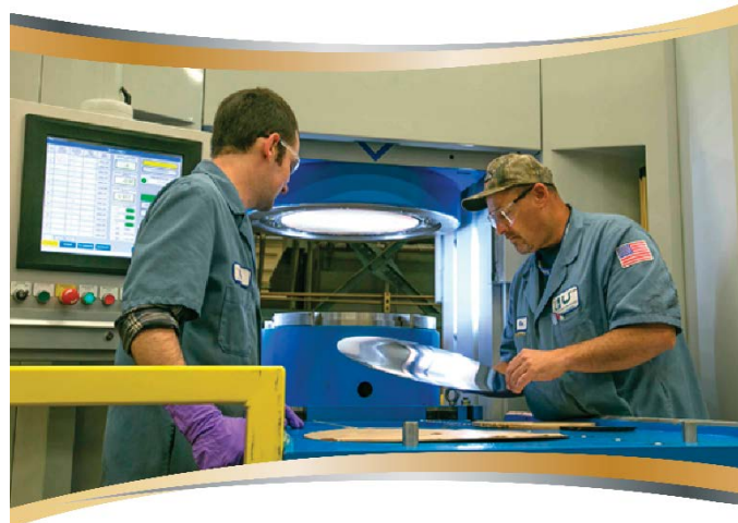
Machinists at Lawrence Livermore National Laboratory use a state-of-the-art hydraulic press needed for W80-4 work. (Photo provided by NNSA)
