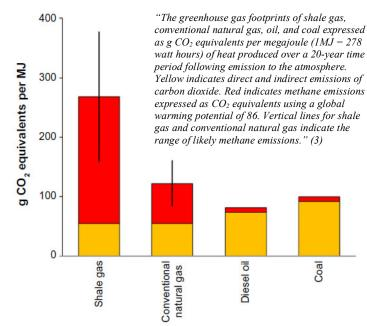
• Methane emissions are comprised of intended and unintended emissions that occur in all parts of the natural gas life cycle. Emissions sources include active wells, aging and dormant wells, refining processes, transportation, and distribution. Intentional venting practices also waste this dwindling natural resource. (6)
