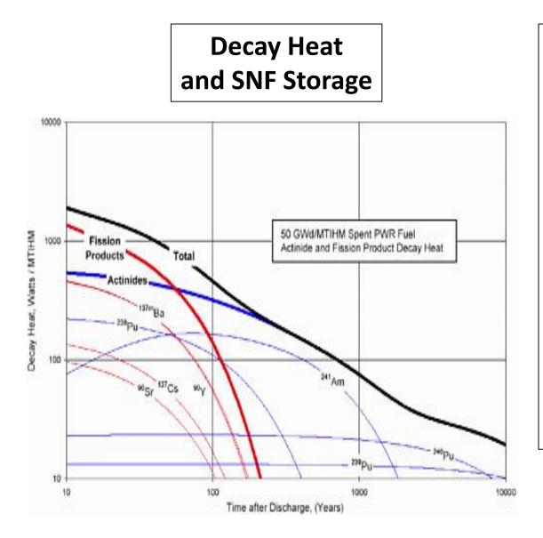
After removal, the spent fuel gives off a significant amount of heat as the radioisotopes decay.
