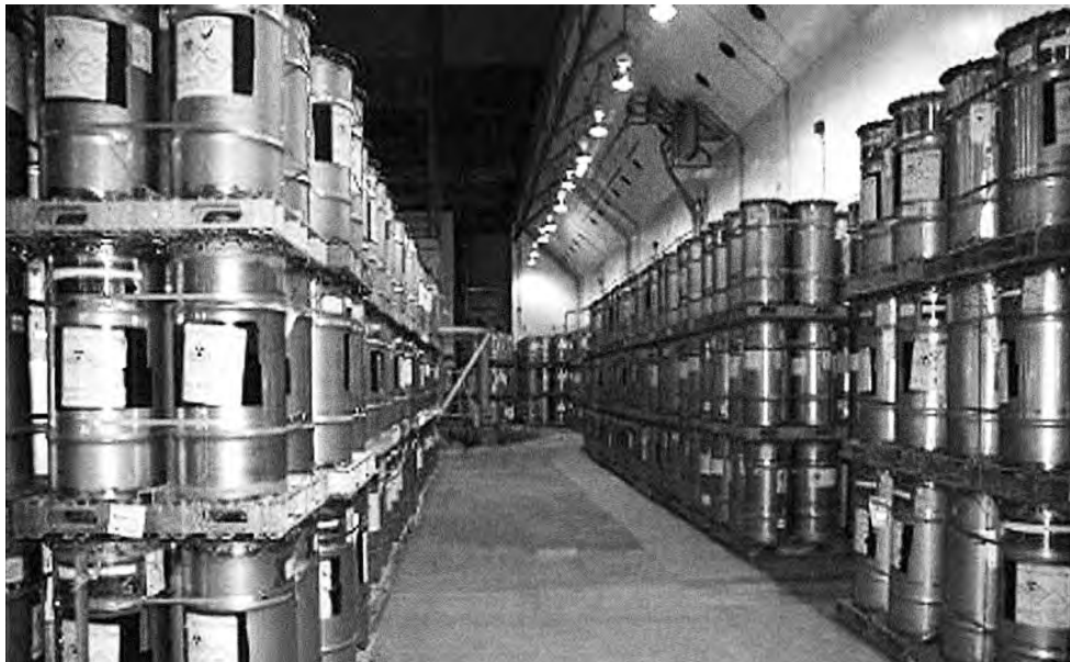
Figure 7 Plutonium storage containers in the U.S. DOE's Savannah River Site K-Area Material Storage Facility where approximately 13 tons of U.S. excess plutonium are stored. Each storage container is about 0.9 meters high and 0.5 meters in diameter and contains up to 4.4 kilograms of plutonium. In addition to protecting the small cans of plutonium within, the outer containers are large enough to prevent a fission chain reaction involving the contents of neighboring cans. 106 Source: H. Allen Gunter, Senior Technical Advisor and Assistant Manager, Nuclear Material Stabilization Project, Savannah River Operations Office, briefing to the Citizens Advisory Board Nuclear Materials Committee, 28 April 2009.
