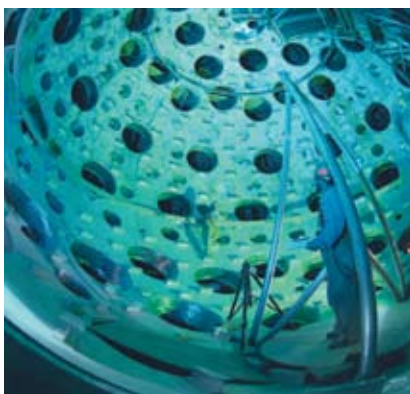
Figure 4.12 A Technician Examines the Target Chamber of the National Ignition Facility During Construction
