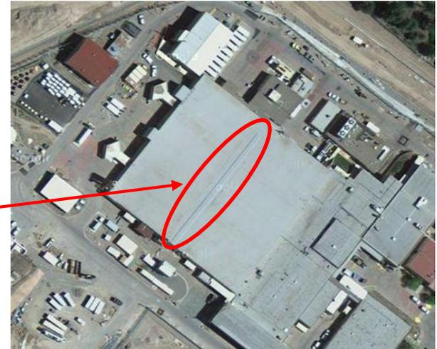
Photo: Google Maps. Photo shows PF-4 roof with drag strut circled.
