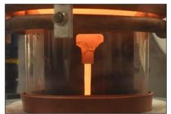
Molten Plutonium in Cast
