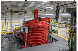
The Multi-Zone Direct Cast Vacuum Induction Melt Furnace at the Testing and Demonstration Facility
