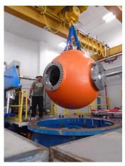
A hydrodynamic experiment confinement vessel being inserted within the DARHT Weather Enclosure
