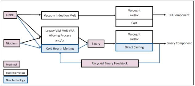
Figure 3–1. Potential production process with new technology insertion
