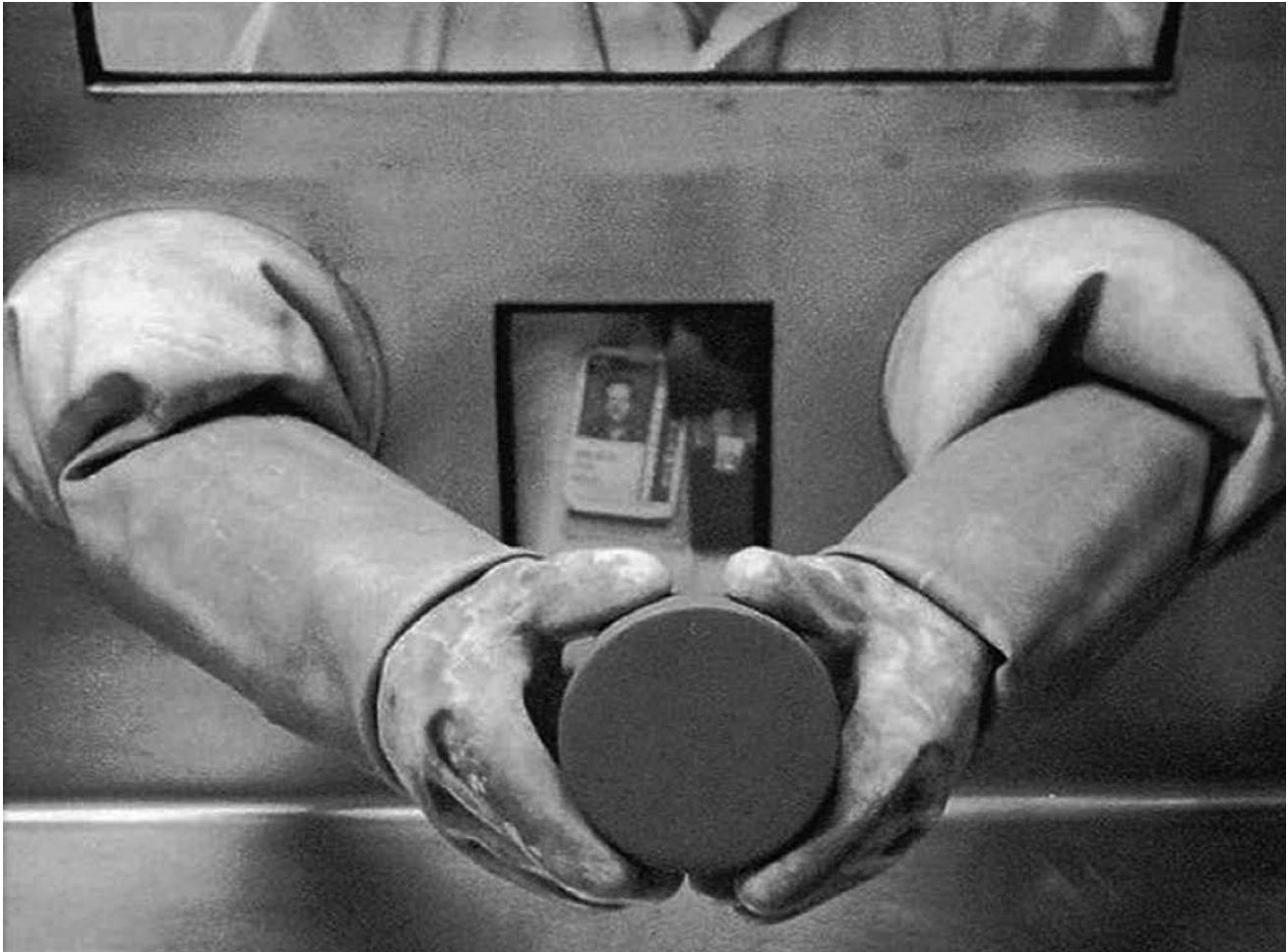
Nuclear materials are often handled in glove boxes such as this to protect the workers.
